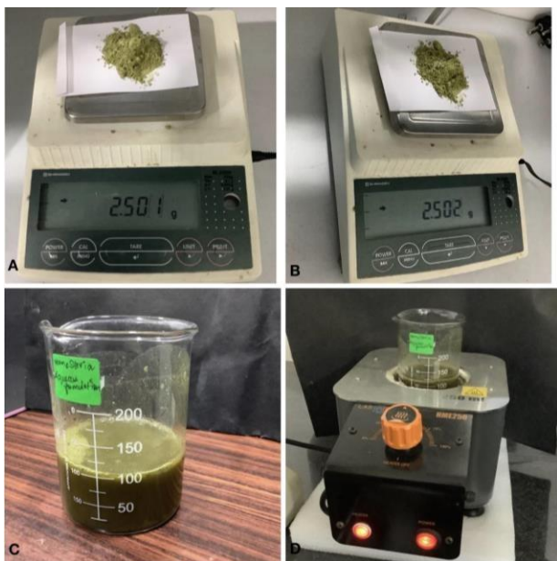
Figure 1: Image A representing 2.5gm of Stevia was measured under the weighing machine. Image B representing 2.5gm of Neem was measured under the weighing machine. Image C representing the Neem and Stevia aqueous formulation and Image D representing aqueous extract of Neem and Stevia boiled for 10-20 minutes at 60 degree Celsius.
