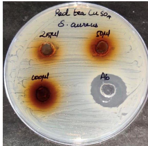
Figure 5: Zone of inhibition of red tea medicated copper nanoparticles by disk diffusion method showing anticariogenic activity against S. aureus .
