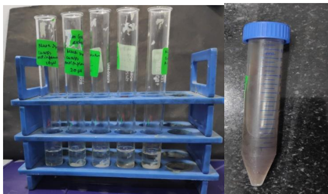
FIGURE 2: The pictures showing the preparation of copper nanoparticles and the collection of pellets of copper nanoparticles after incubation.
