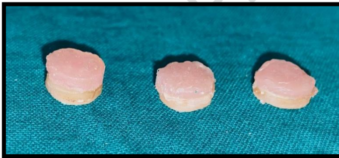
Figure 3- soft liner bonded to acrylic resin
