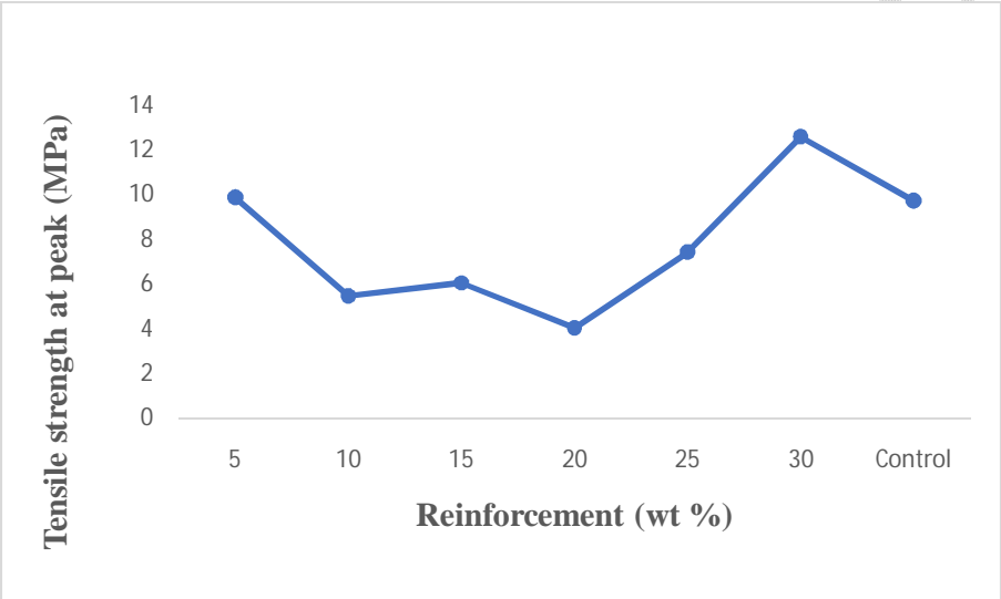
Figure 5. Variation of tensile strength at peak (MPa) with the composite and control
