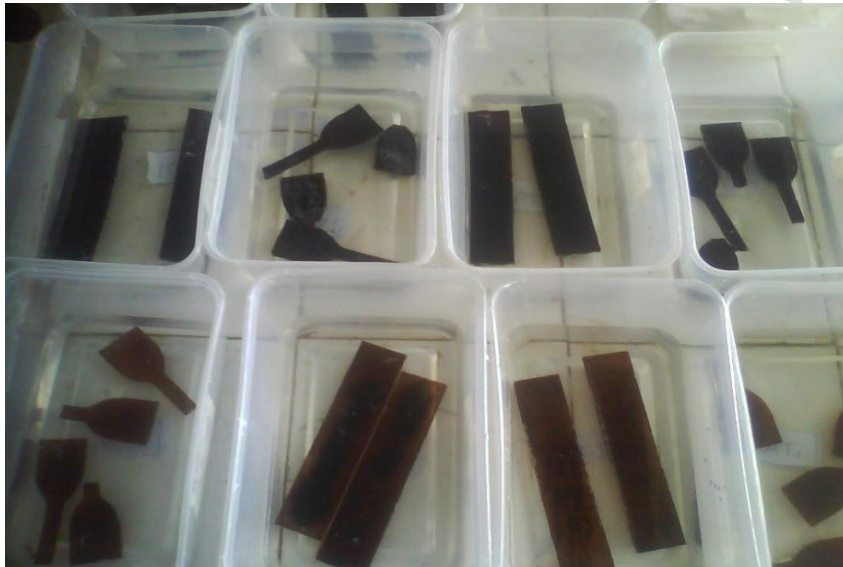
Figure 3. Water absorption test
