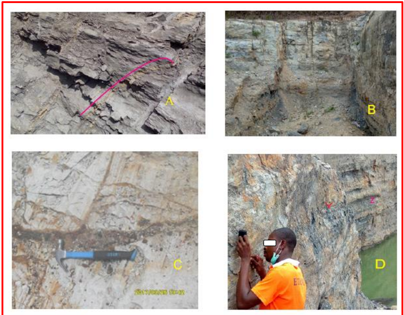
Figure 7: Fracture occurrences at the sandstone zones. (a) curved fracture at the shale, (b) long trending vertical fractures, (c) T-junction fracture, (d) terminating fracture at Uburu.
