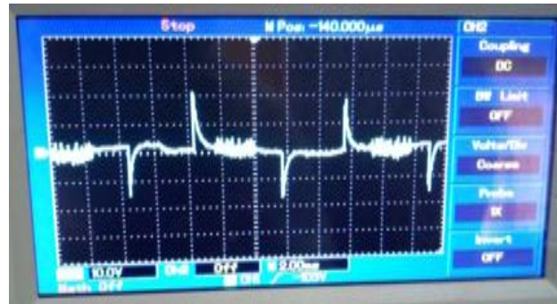
Fig. 13 Inductive load voltage profile of the hybrid super-capacitor/battery storage system
