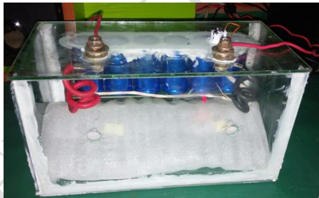
Fig. 3 A super-capacitor bank rated 16.2V,83.33F.
