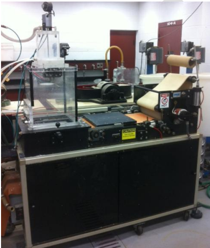
Fig. 3. MK Systems Inc. dynamic sheet former [25]
