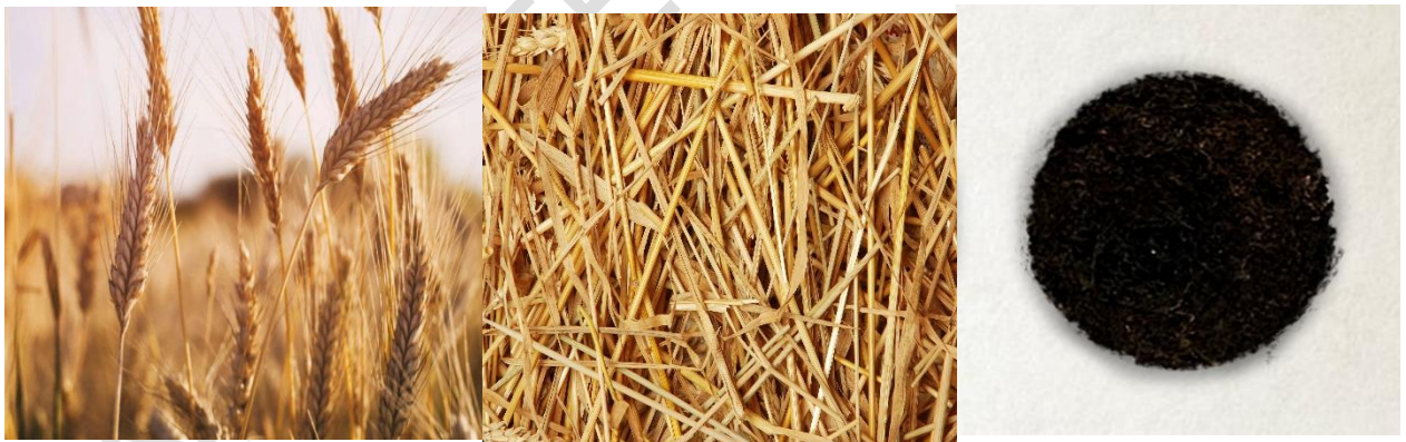
Figure-2 a) Wheat crop b) Wheat Straw separation c) Wheat straw ash burning at 800°C for 30min
