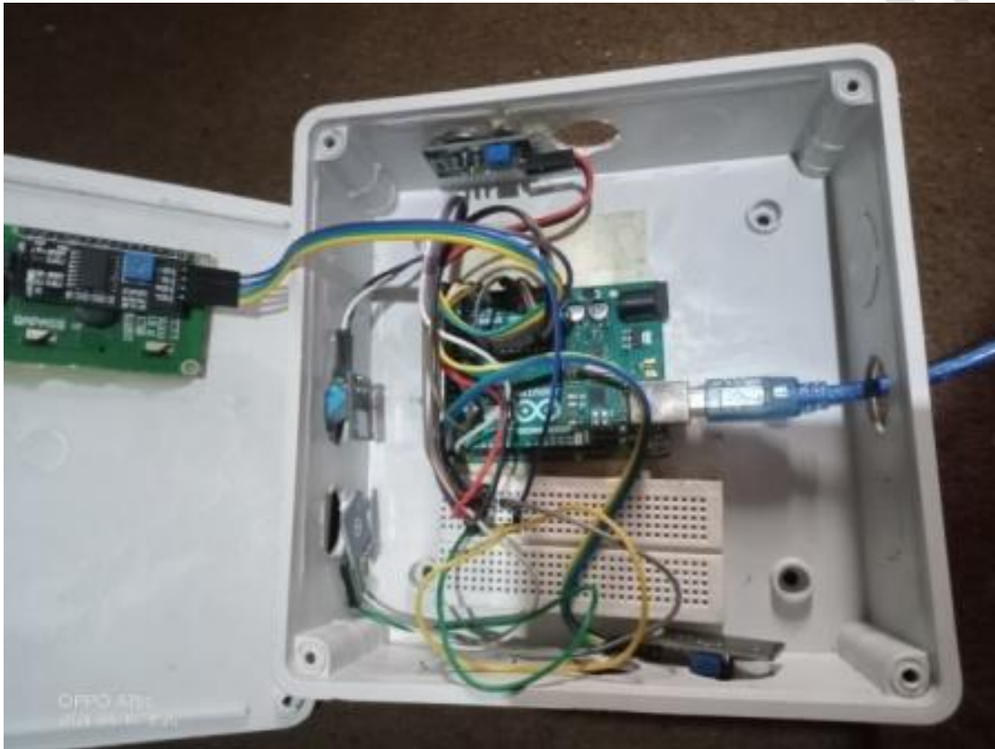
Figure 4.1: Components arrangement in the Adaptable box
