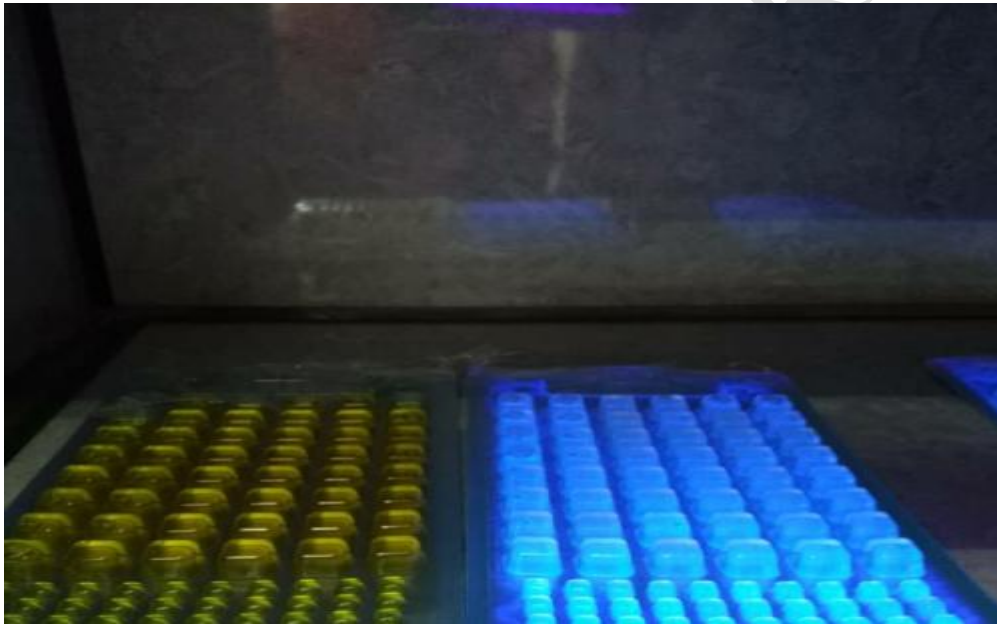
Fig 2: Negative and positive results of bacterial growth after exposing colilert and Pseudalert test to UV
