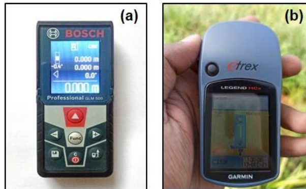
Fig.2. (a) Laser rangefinder (Bosch Glm 500 Laser Distance Measurement Device), (b) Geographical Positioning System (GPS)
