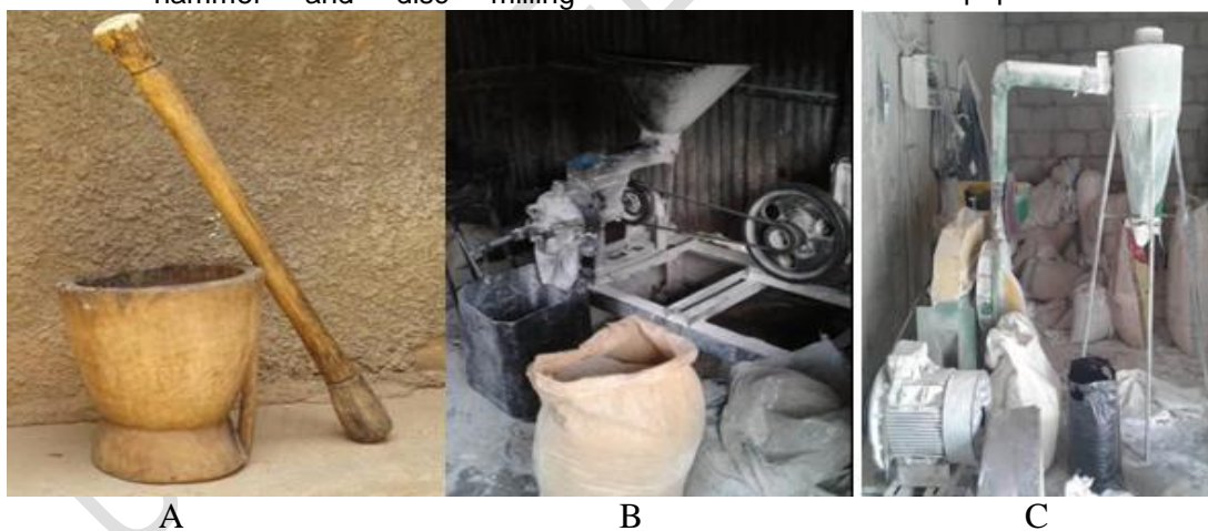
Figure 2: Grinding methods: (A) mortar and pestle; (B) Hammer mill and (C) Disc Mill.
