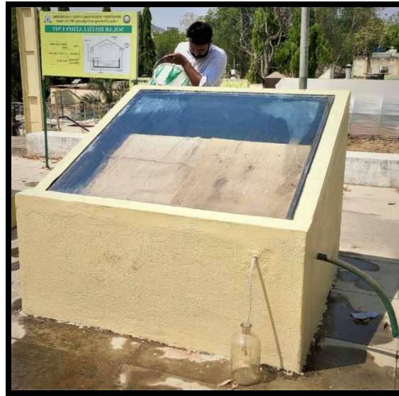
Fig.1. Developed Passive solar distillation unit
