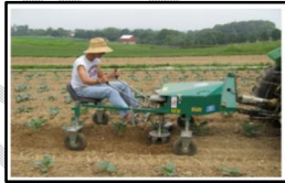
Fig.3: ECO weeder requires an operator to move rotating weeding mechanisms with tines (HCC. 2011)
