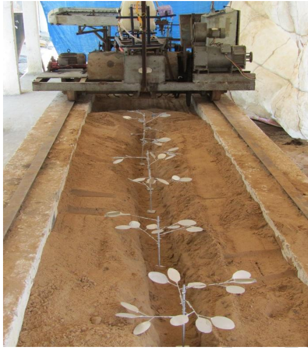
Plate 3: Experimental setup to study effect operational parameters on droplet size of the nozzles on artificial plants.
