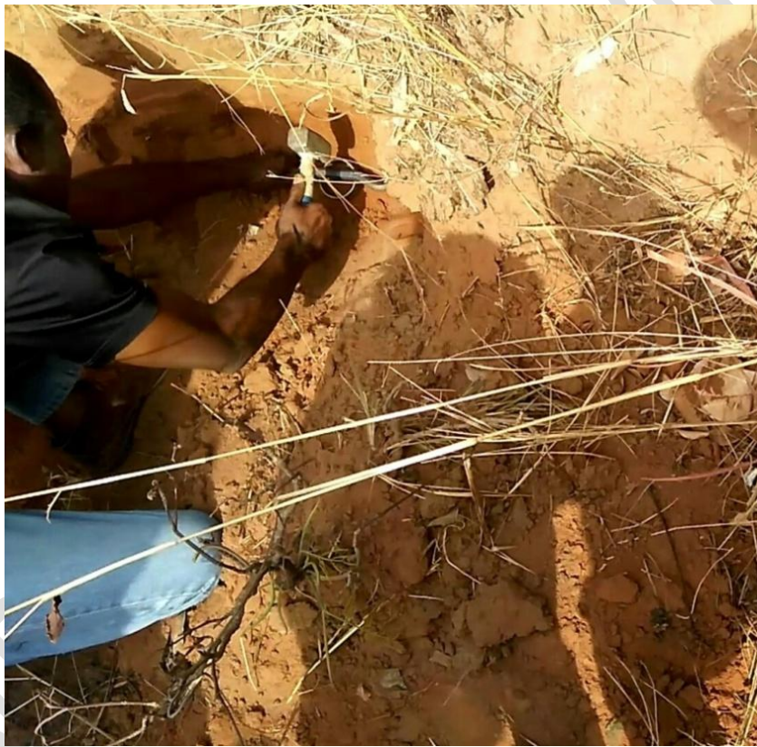
Fig 5a: Extracting Soil Sample with Core
