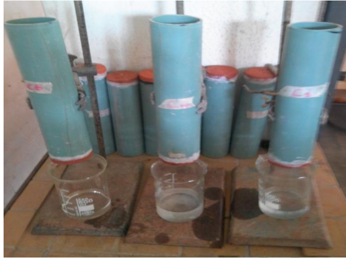
Figure 3: Experimental set up for filtration rate test
