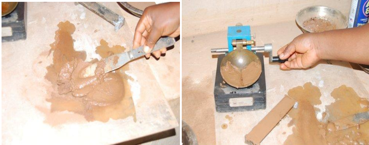
Fig. 13: Atterberg limit test in progress.
