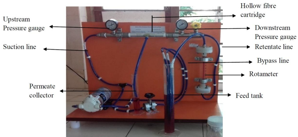
Plate 1Hollow fibre membrane setup
