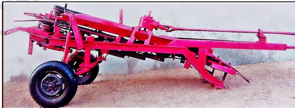
Fig. 4: Developed harvesting machine for onion crop (Nour et al., 2020)
