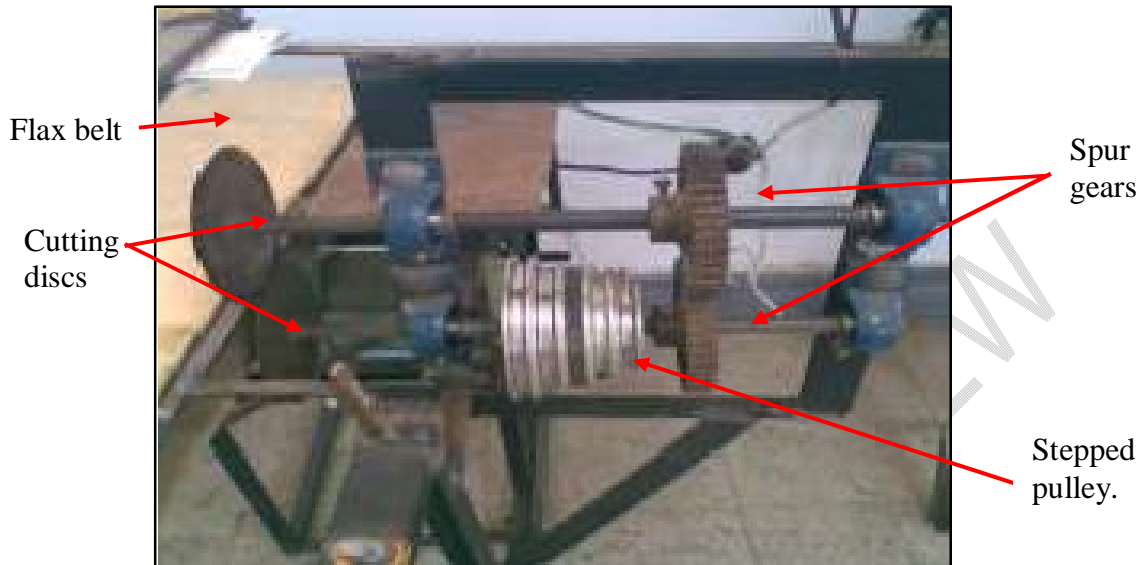
Fig. 6: Trimming unit of green onion crop handling mechanism (Mayhoub et al., 2009)
