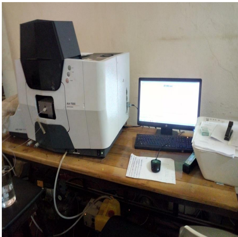
Plate 1: Front view of the atomic absorption spectrophotometer with the monitor and printer.
