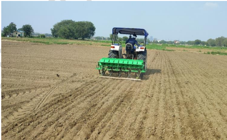
Fig. 2 Direct seeding of rice with tractor drawn DSR planter
