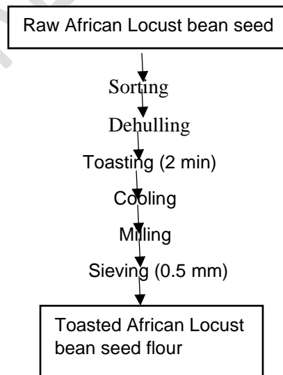
Figure 5: Flow chart for the production of toasted locust bean flour (Ogunsina et al., 2015) slightly modified
