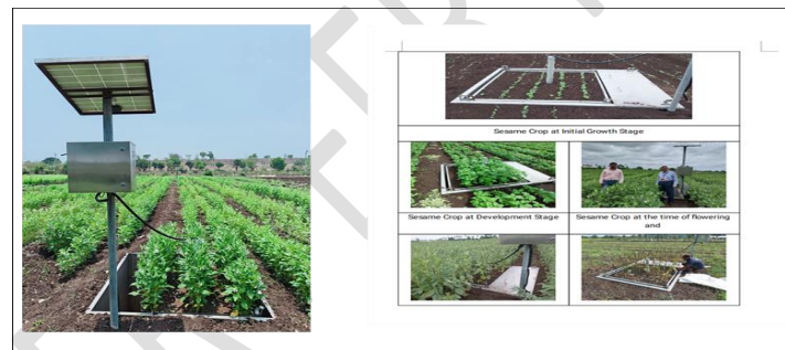
Fig 2 Digital weighing lysimeter for estimation of Crop Evapotranspiration
