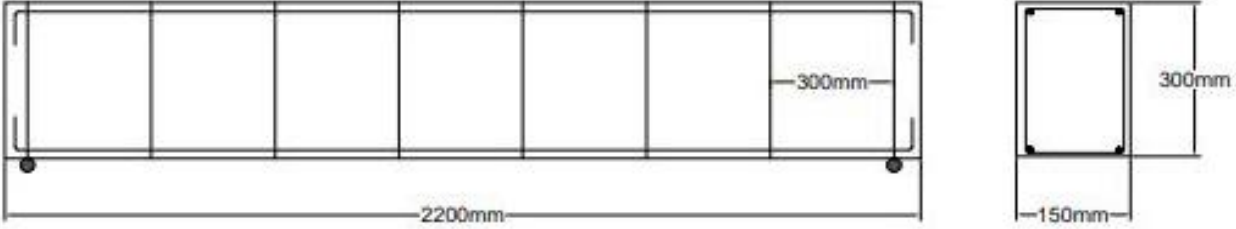
Fig. 3(a). Illustration of control solid beams (B1 and B7) without any opening and PVC pipe.
