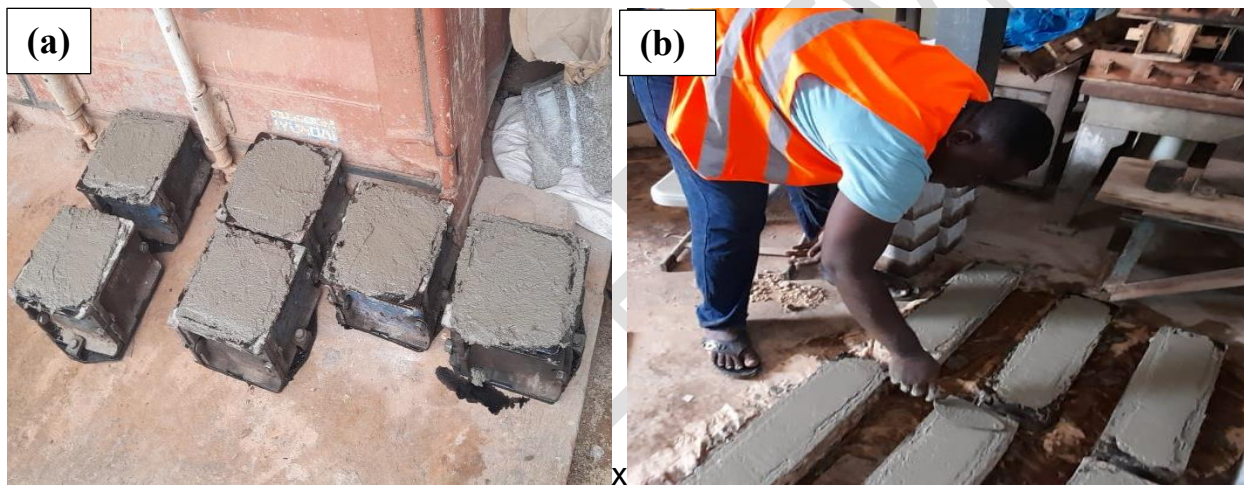
Fig. 2. Specimens: (a) concrete cubes, (b) concrete prisms
