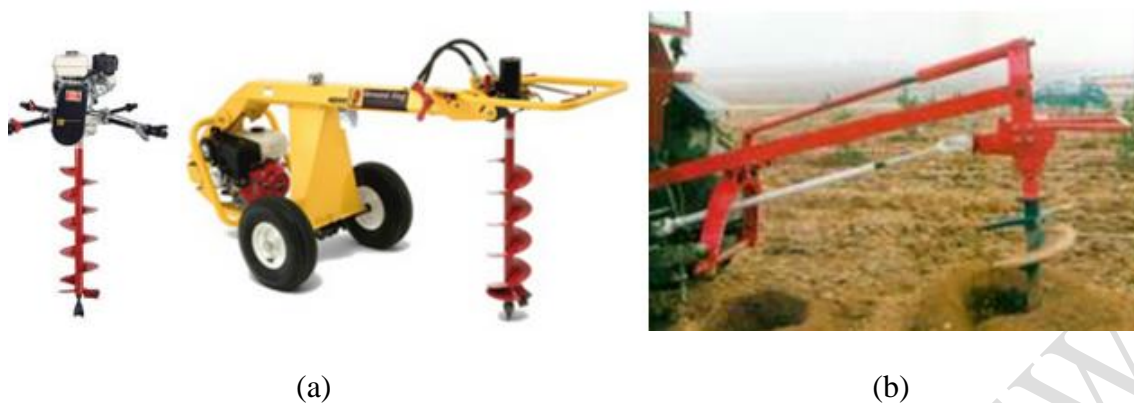
Fig. 4. Pit hole diggers (a) motorized and (b) tractor-operated for digging pits for litchi planting
