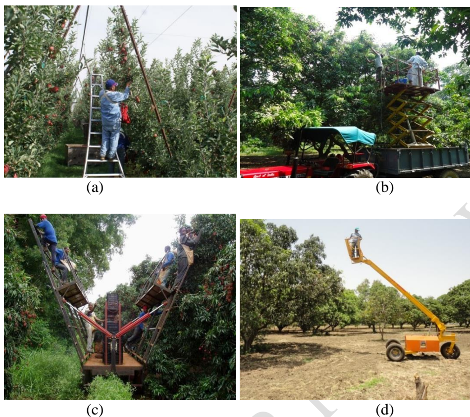
Fig. 11. Harvesting aid for litchi (a) harvesting ladders, (b) tractor-operated hydraulic platform, (c) hydraulic operated ladder, and (d) self-propelled hydraulic platform
