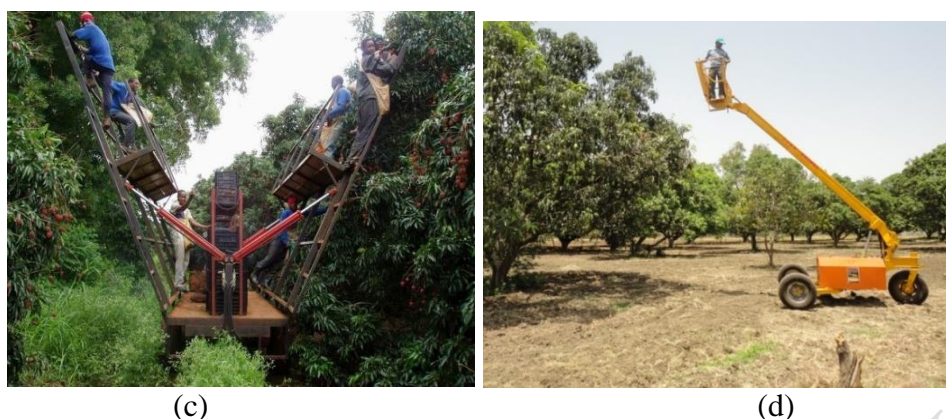
Fig. 11. Harvesting aid for litchi (a) harvesting ladders, (b) tractor-operated hydraulic platform, (c) hydraulic operated ladder, and (d) self-propelled hydraulic platform
