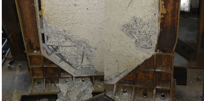
Fig3 Failure mode of SRCW specimen
