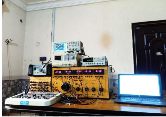
Plate 1: HIL Set-up for Running the Taguchi L9 Orthogonal Array Experimental Levels
