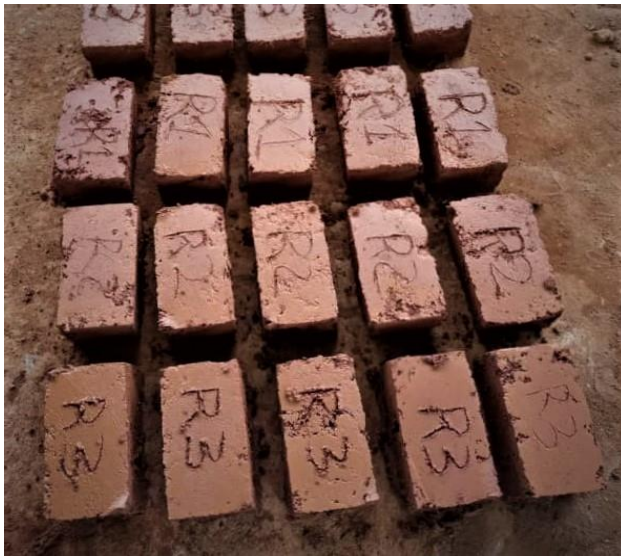
Fig. 2. (a.) freshly moulded block specimen
