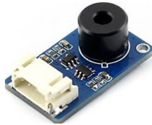
Fig. 3 Contactless Infrared (IR) Temperature Sensor Unit (Waveshare 2023)
