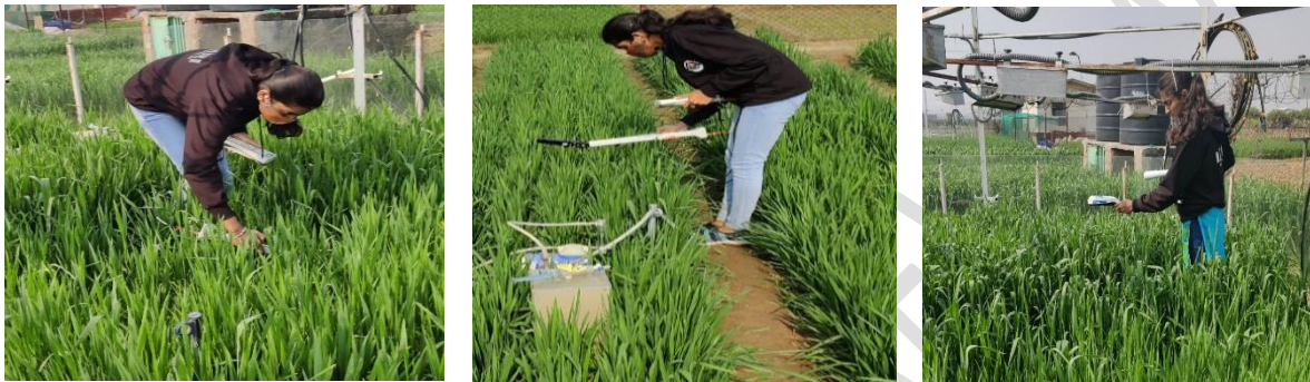
Fig 3: Using the canopy analyser and green seeker at Genetic-H field, IARI-New delhi
