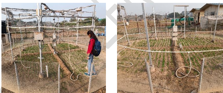
Fig 2: wheat crop grown in T-FACE facility at Genetic-H field, ICAR-IARI, New Delhi
