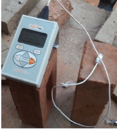
Figure 2: Photo of KD2 Pro device
