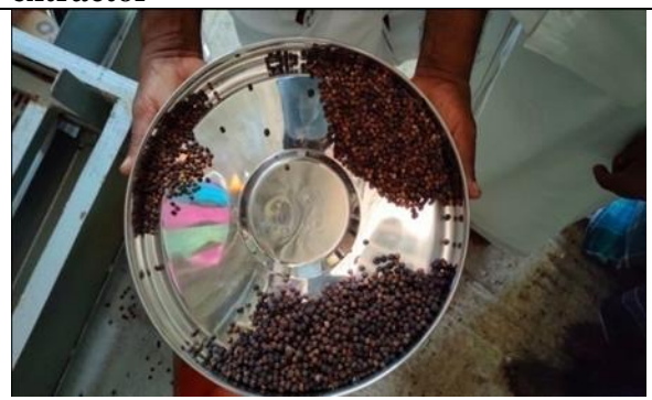
Fig.6. Graded pepper by using pepper grader
