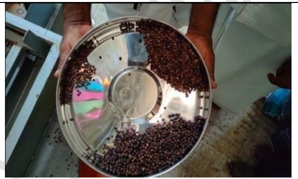
Fig.6. Graded pepper by using pepper grader
