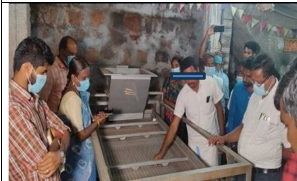
Fig.5. Pepper grading by Pepper grader
