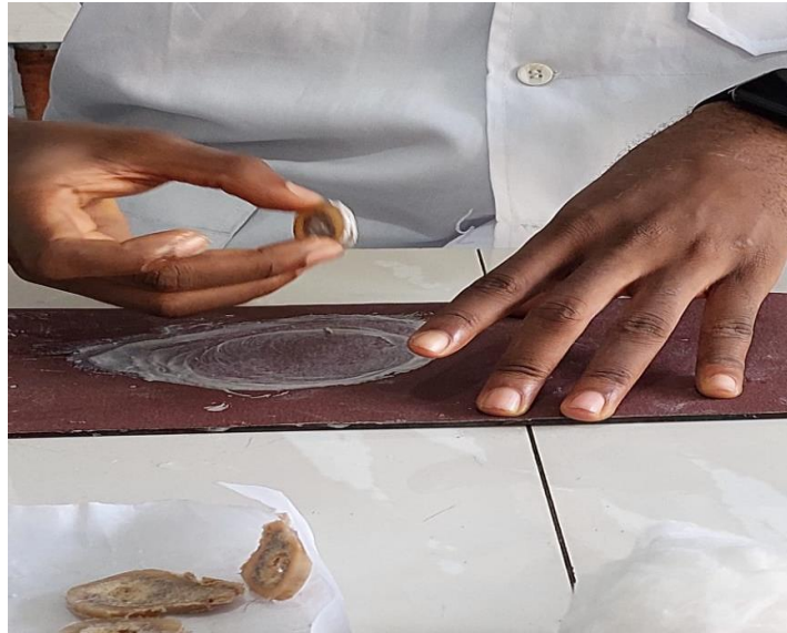
Fig.2. The investigator grinds a section of the femur bone using the Modified Frost Manual method
