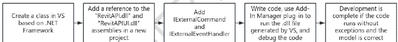
Figure 1. Revit secondary development process
