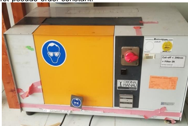
Fig.1. Experimental setup used for photodegradation of MB
