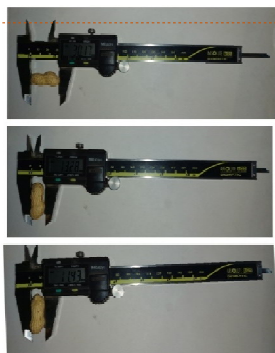
Fig.1: Measurement of size of groundnut pods
