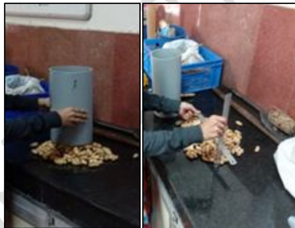
Fig.4: Determination of angle of repose of groundnut pods
