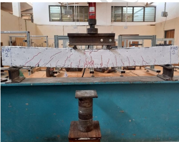
Fig 3: Beam Specimens during and after testing.
