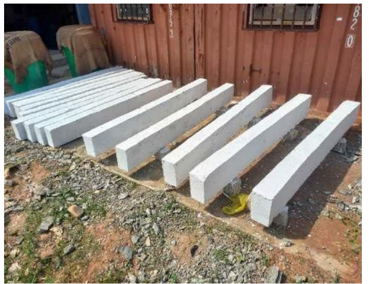
Fig.2: Preparation of Reinforced Concrete Beam Specimens.
