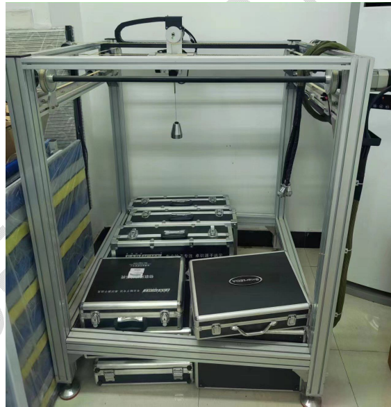
Fig. 1. Experimental equipment of the 3D bridge crane
