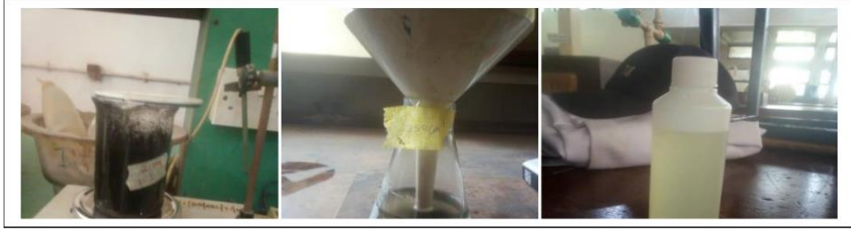
Plate.1 : Preparation of leach liquor
