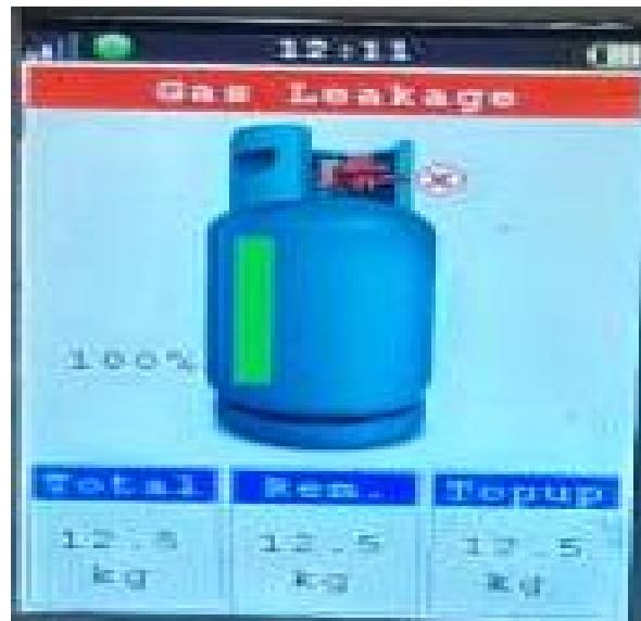
Figure 12: Gas leakage notification via LCD
