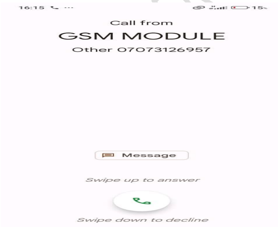
Figure 9: Incoming call drawing user's attention to gas leakage
