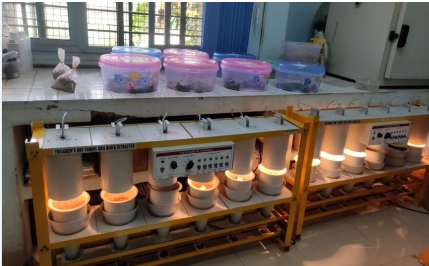
Plate 2: Setting of Berlese Funnel for the Estimation of Soil Invertebrate population from collected samples
