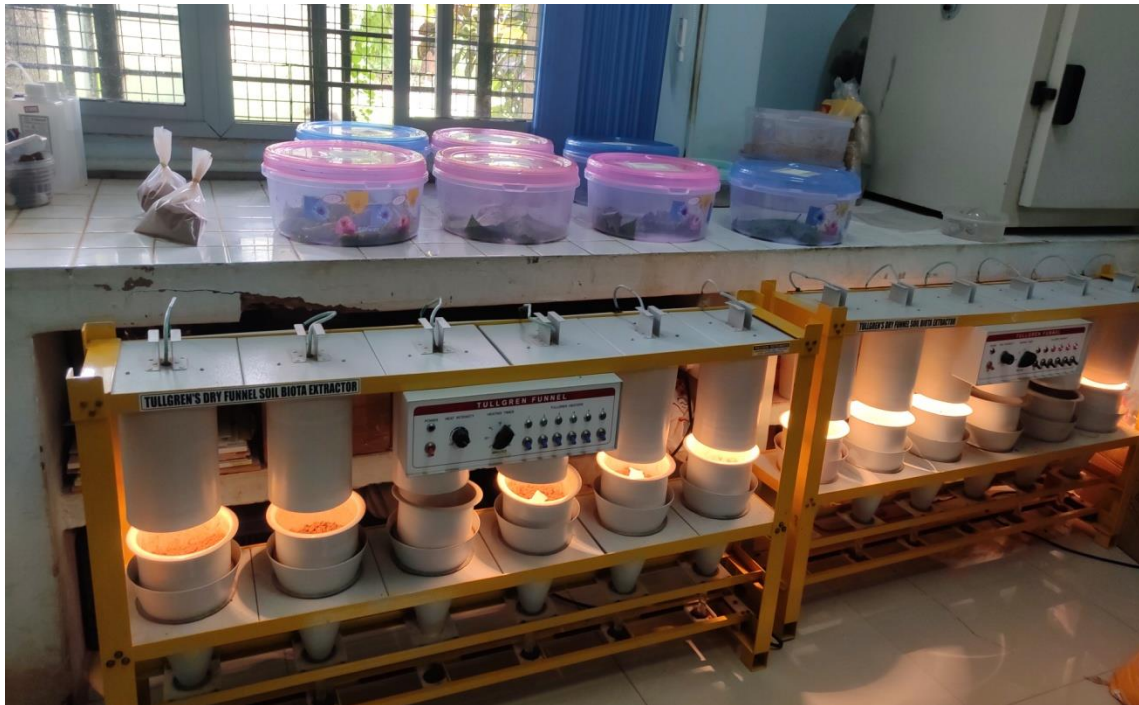
Plate 2: Setting of Berlese Funnel for the Estimation of Soil Invertebrate population from collected samples
