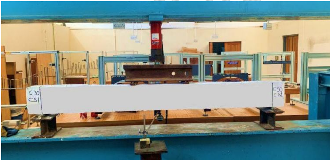
Fig. 2. Beam testing set-up
