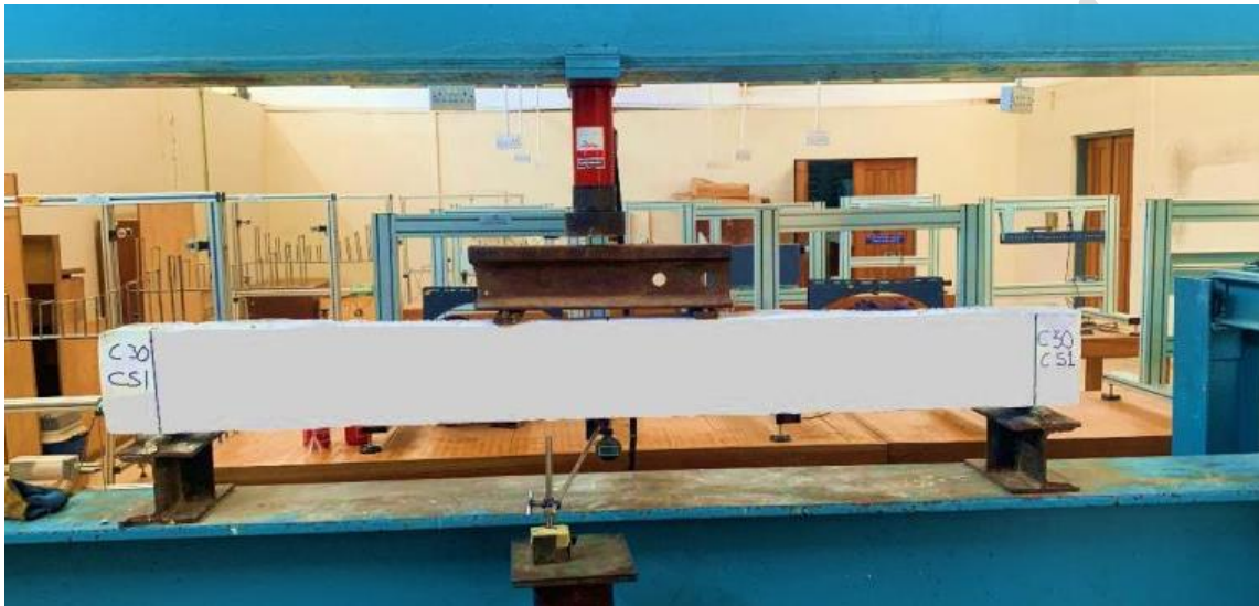
Fig. 2. Beam Testing set-up
